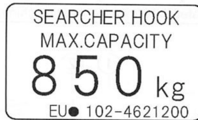
(2) Searcher Hook Maximum Gross Rated Total Load (102-4621200)
