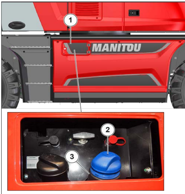
Figure 149: Checking DEF liquid level
