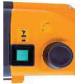
Green start button and key switch
